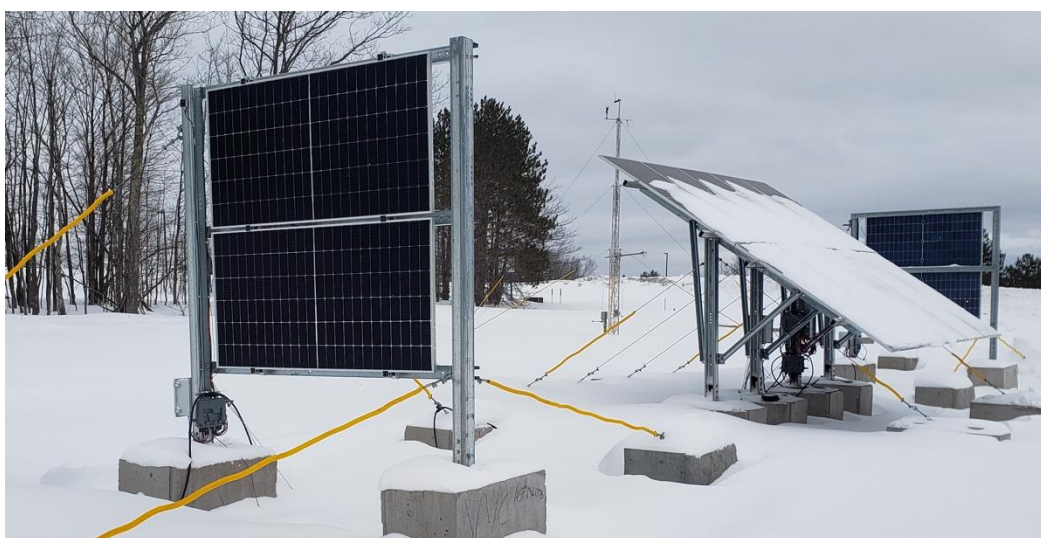
Figure 19: Example of a hybrid orientation system installed by Sandia National Laboratories at the Michigan RTC. Analysis is underway of the relative performance of the south-facing fixed-tilt vs vertical east- and west-facing bifacial modules, which collect almost no snow. Photo credit: Paul Dice .
