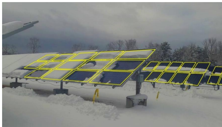
Figure 20: Snow accumulation on PV modules with a single-axis tracker. The yellow quadrilaterals indicate the segmentation of the modules for analysis of non-uniform shedding patterns. Photo Credit: Laurie Burnham.
