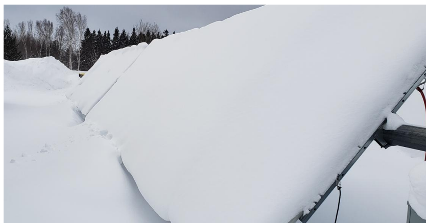
Figure 15: Heavy snow load on a tracker system at the Michigan Regional Test Center (RTC), combined with high snow depth and some drifting, have rendered this system temporarily inoperable. Photo credit: Paul W. Dice .
