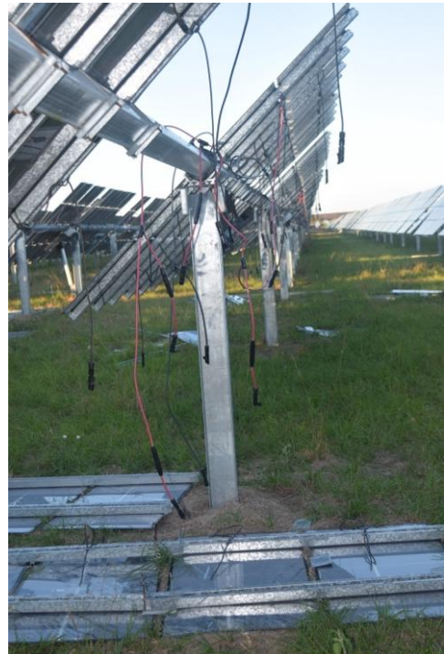
Figure 6: Tracker system damaged by Hurricane Helene in the US in 2024 is shown here. Fastener failures caused modules to detach from the torque tube and tear from electrical connections.
